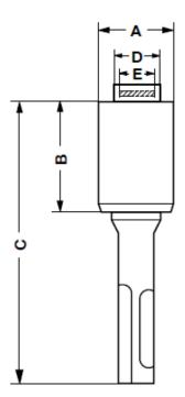
**Nail attachment** with SDS adaptor to be fitted in a percussion power tool. A magnetic disc on front side provide nail catching for a quick and easy riveting.
